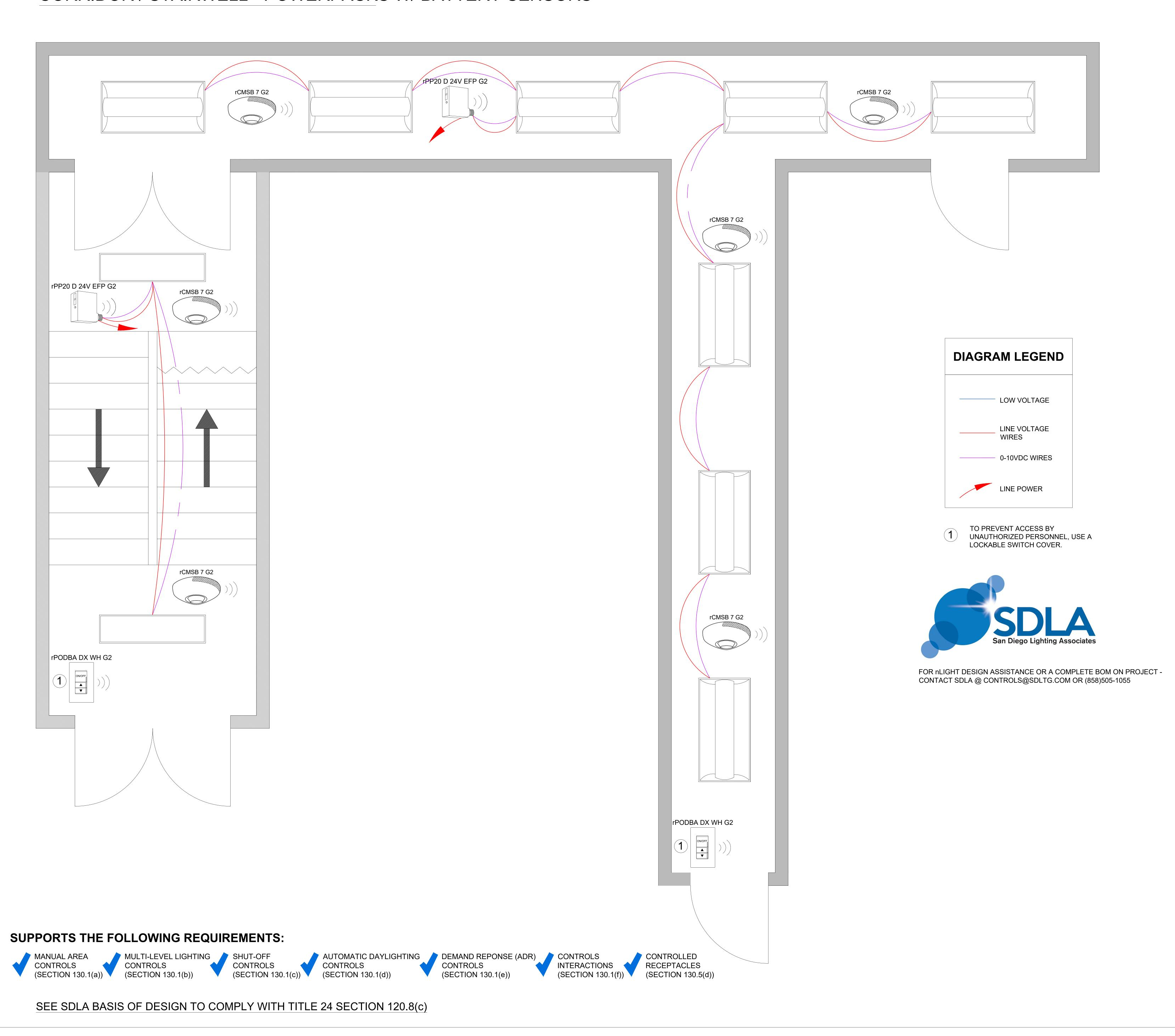
nLIGHT AIR: CORRIDOR / STAIRWELL - POWERPACKS W/ 24VDC SENSORS
